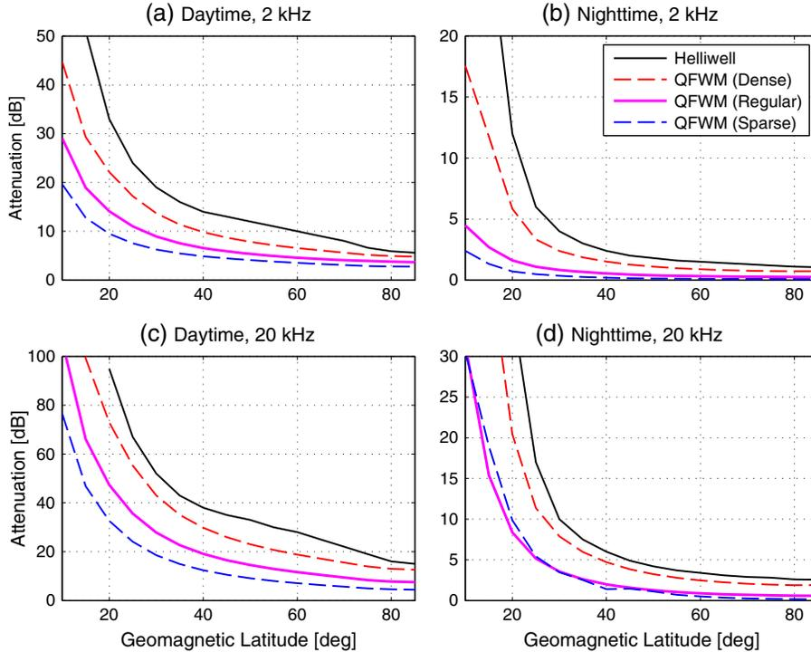
**Figure 7.** Estimates of trans-ionospheric attenuation of a VLF whistler-mode plane wave vertically incident upon the ionosphere. Results are provided for (a) daytime, 2 kHz; (b) nighttime, 2 kHz; (c) daytime, 20 kHz; and (d) nighttime, 20 kHz. Dense ( $\times 2$  daytime,  $\times 5$  nighttime), regular (see Figures 1c, 1d, 2c, and 2d), and sparse ( $\div 2$  daytime,  $\div 5$  nighttime) ionospheres are considered for each case. Helliwell’s absorption curves are included for reference.
