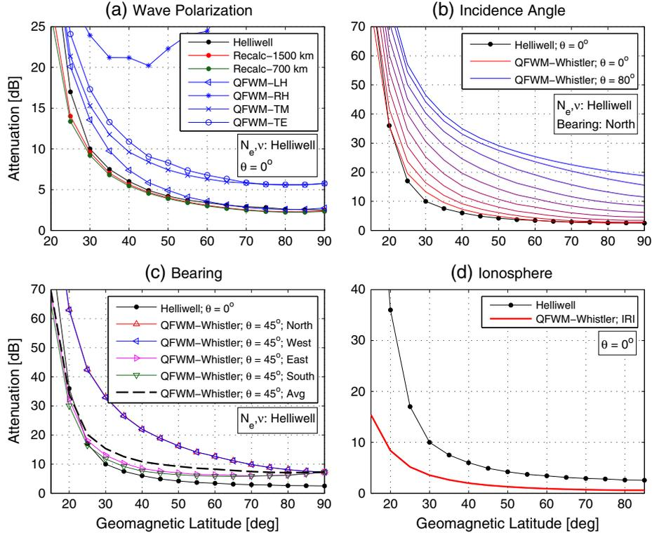
**Figure 3.** Illustrative QFWM results showing the importance of various factors which affect trans-ionospheric attenuation of VLF waves: (a) wave polarization, (b) incidence angle, (c) bearing, and (d) ionosphere profile. All curves are for a 20 kHz wave at nighttime. Helliwell’s absorption curve is included as the dotted black curve in each panel, and our recalculation of Helliwell’s absorption curve is included in Figure 3a.
