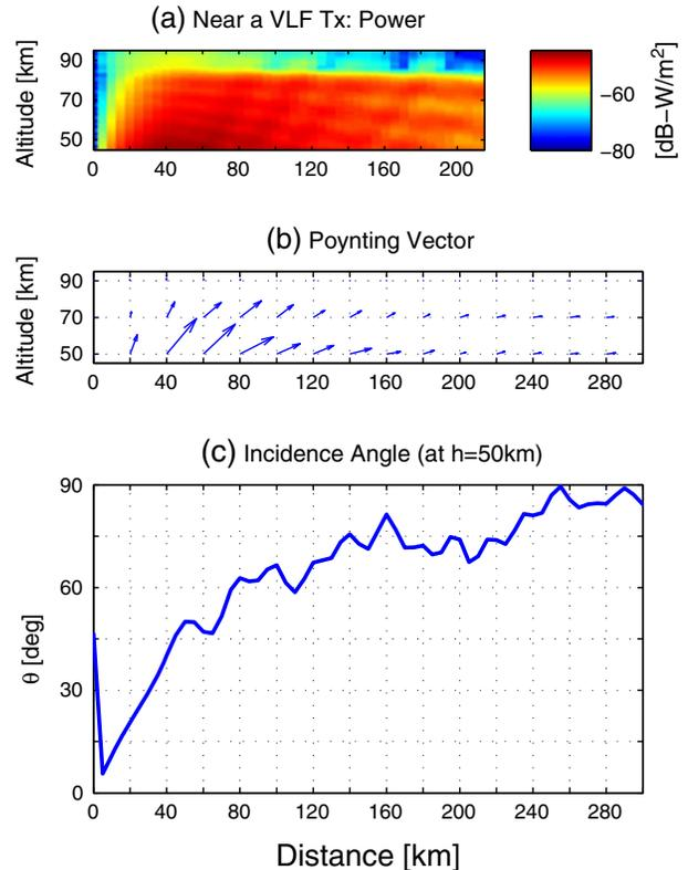
**Figure 8.** (a) Illustrative FWM results depicting (b) the direction and relative magnitude of the Poynting vector near the base of the ionosphere in the vicinity of a terrestrial VLF transmitter. (c) The estimated wave incidence angle, which very quickly approaches grazing incidence as the wave progresses forward in the Earth-ionosphere waveguide.
