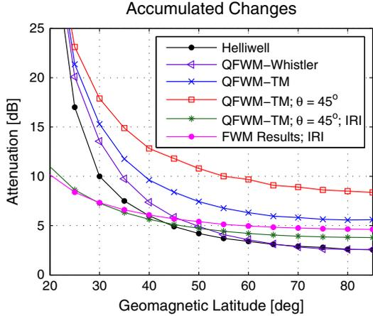
**Figure 4.** Accumulated changes to the trans-ionospheric attenuation of a 20 kHz wave at nighttime, illustrated using QFWM results. The effects of polarization, incidence angle and bearing, and updated ionosphere profiles are sequentially added. Also shown are Helliwell’s absorption curve in dotted black and the FWM results in dotted magenta.
