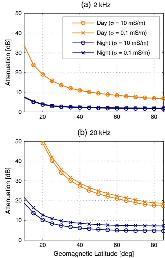
**Figure 6.** Comparison of FWM trans-ionospheric attenuation estimates for different values of ground conductivity. Results are provided for (a) 2 kHz and (b) 20 kHz, and for daytime (orange) and nighttime (blue). Results for  $\sigma = 0.1$  mS/m are marked with circles, and results for  $\sigma = 10$  mS/m are marked with x's. We use the ionosphere profiles of Figures 1c, 1d, 2c, and 2d for each curve.
