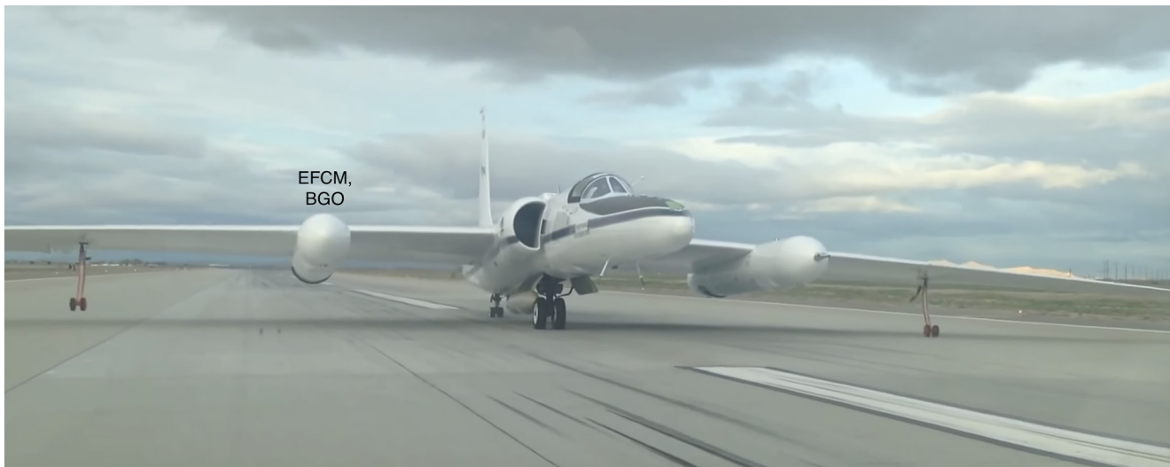
Figure 1. The ER-2 Airborne Lightning Observatory for FECS and TGFs (ALOFT). The electric field change meter (EFCM) and the gamma-ray detectors (BGO) are located inside the right pod. The image is from (Tatum, 2017). ALOFT, Airborne Lightning Observatory for FECS and TGFs; BGO, bismuth germanate; EFCM, electric field change meter; FECS, Fly's Eye Global lightning mapper Simulator; TGF, Terrestrial Gamma-Ray Flash.
