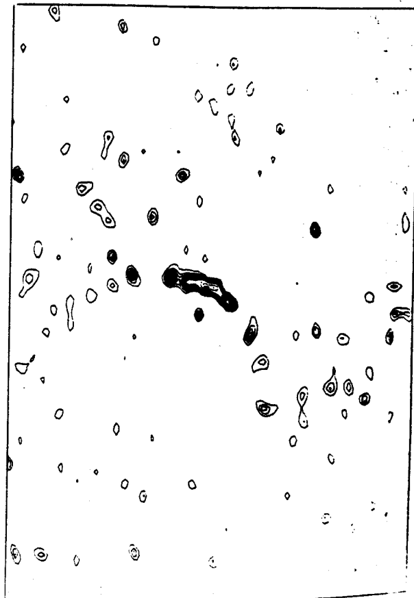
Fig. 3 An example of the mis-use of the maximum-entropy method. The spurious features, which are not present in Fig. 2 b , result from an over-optimistic estimate of the noise level in the data.
